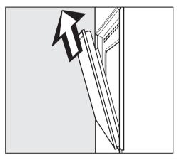
■ Hold the door securely at both sides and lift upwards off the hinge guides.
